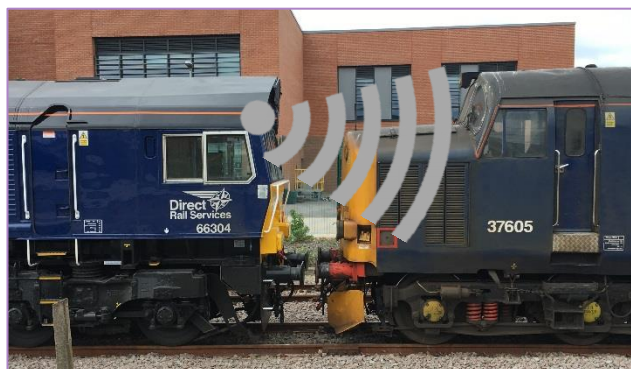
Figure 1 Positioning of FFCCTV camera
